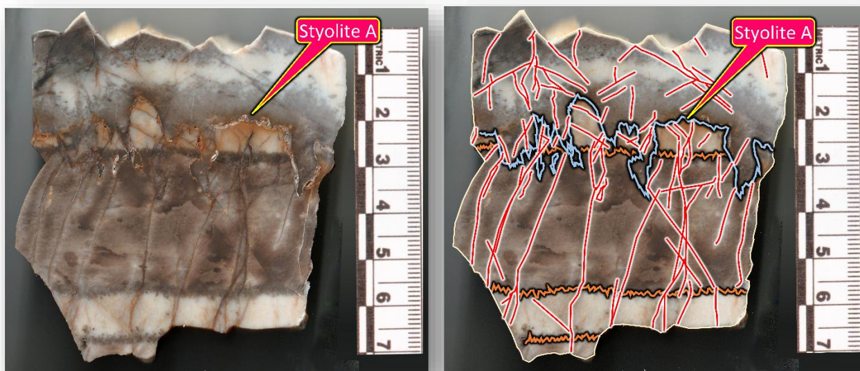
Figure 14. Sample 1 was sawed, sanded and then scanned. Styolites and fractures interpreted on the second image. Observe that there are small styolites (orange) and a later larger styolite, Styolite A (blue). This one cuts the earlier small ones and represents a larger amount of dissolution. Many fractures are highlighted in red. Beneath Styolite A are a series of fractures at high angles to the styolites. Similar fractures are not observed in the section above Styolite A. Above Styolite A, the novaculite presumably had slightly different properties in terms of its ability to transmit fractures.
